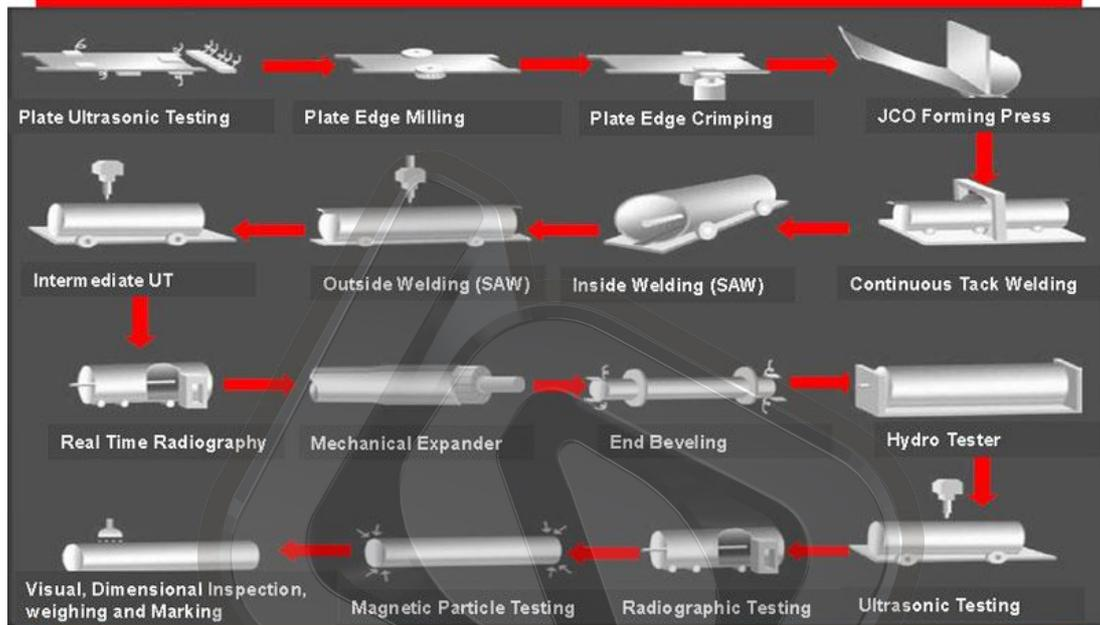
Production Process of LSAW pipes
