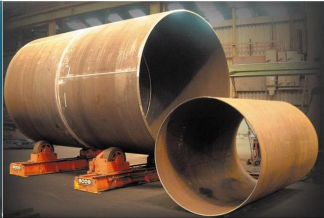
2m pipe segments welded together(big diameter)
