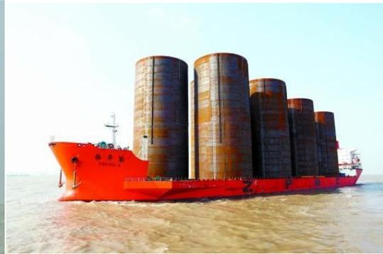
China South Sea Project Diameter:21m Length:85m Weight:705tons/pipe
